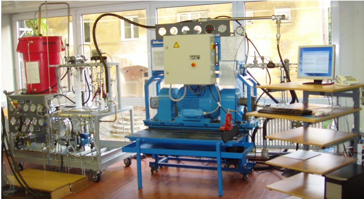
Figure 3: Water hydraulic test rig on the left-hand side and the oil hydraulic test rig on the right-hand side [7]
